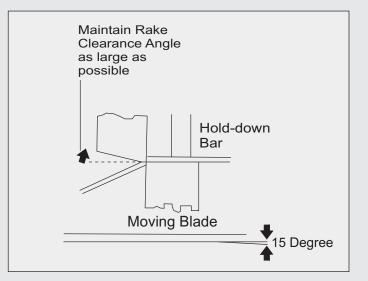
The most suitable shear blades for cutting 409M and stainless steel are made of high carbon – high chromium tool steel. The blades must be kept sharp – a good test is to cut a piece of paper.
